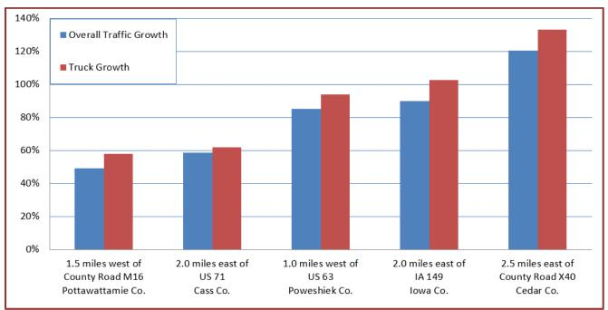
Figure 5. Overall Traffic and Truck Growth from 2014 to 2040
