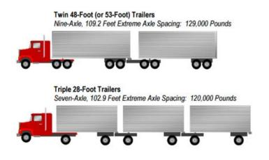
Figure 11. Longer Combination Vehicle Examples
