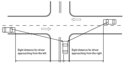
Figure 26: Stopping sight distance (SSD) for access connections.
