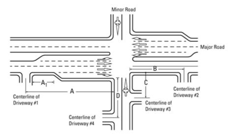
Figure 32: Functional intersection area as a determinant of driveway location
