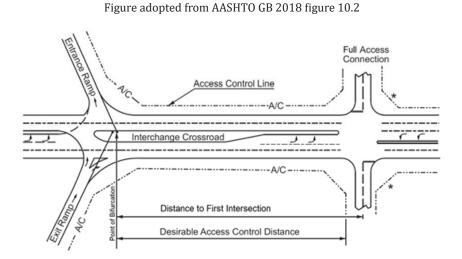
Figure 23: Access control near interchange ramps
