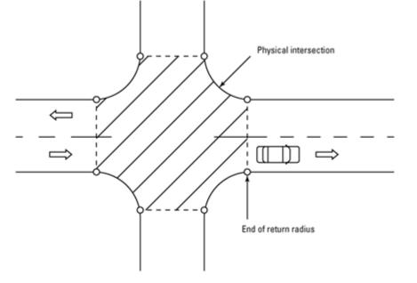
Figure 31: Illustration of when a vehicle has cleared an intersection
