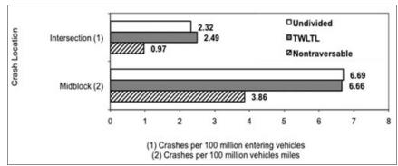
Figure 5: Pedestrian crash rates for suburban arterials.
