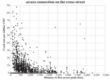
Figure 9: Crash rate per million VMT compared to the distance to the first
