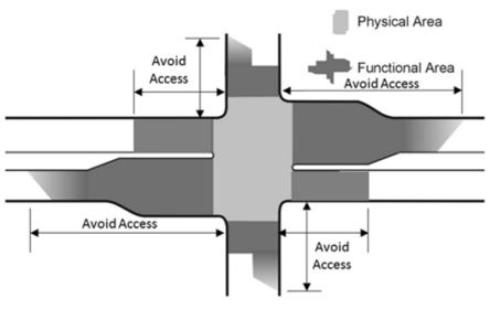
Figure 28: Functional area of an intersection where access should be avoided
